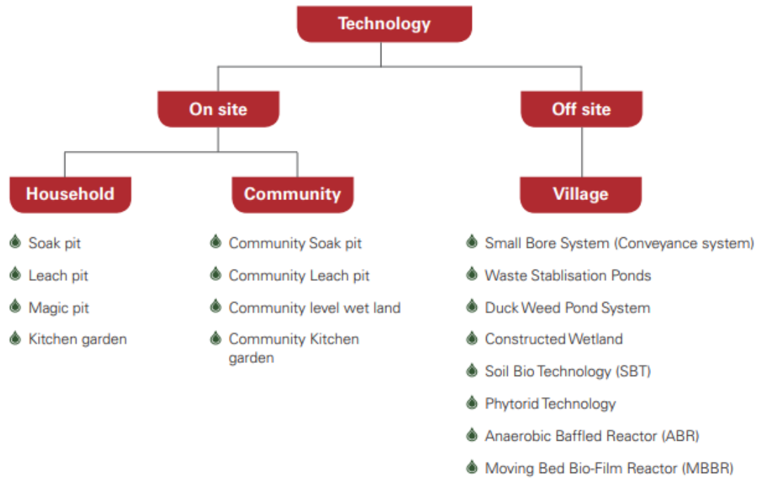
Figure 2.4.1. Technologies available for greywater treatment
