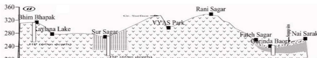
Fig.4.1: Cross-section of the ground in the greater Jodhpur area – the main city is located on the bowl on the right-hand side
