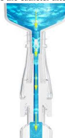
Figure 1.2: Pathway for fluid to pass when the syringe is connected
